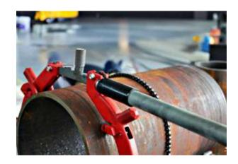
The Macstroc Rotary pipe cutter, designed for extremely low clearance and up to 36-inch pipe diameter, efficiently cold cuts steel, galvanized, and black iron pipes in tight spaces without producing debris, sparks, or significant heat, delivering a precise cut suitable for confined spaces such as trenches, underwater environments, noise-sensitive areas, overhead applications, and pipe racks.
